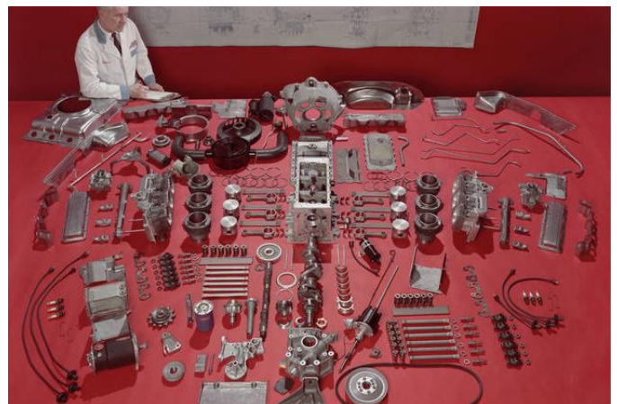
View of a 1960 Corvair flat-six shows the short-stroke crankshaft.
