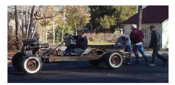
May 2005: The engine was removed from the chassis and overhauled by Jim Linner at Front Range Machine in Longmont. The chassis has been cleaned, with all components rebuilt and/or reconditioned. The assembled and detailed driveline and chassis are ready for the body to be refitted.
