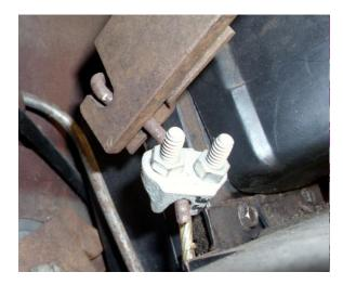
The eyebolt slips into the clutch clevis and the clamp holds the end of the cable. Of course, it helps when the failure is at an exposed end, not under the belly pan.
