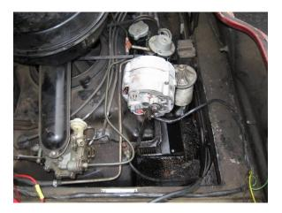
The last mechanical work done in the car was to repair an oil cooler fin leak and install new oil cooler seals. This leak extends as far forward as the left carb area of the seal, and then it pools down to the rear. Some oil appears on the ground beneath the oil cooler area; in addition,
