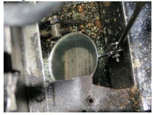
So he drained the oil and removed the cooler. The seals were still quite pliable and you could see that the December epoxy repair had held nicely. The new leak was likely from a split in one of the fins itself.
